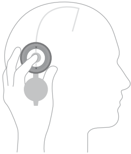
Fig. 9: Localising the valve using the M.blue Compass
